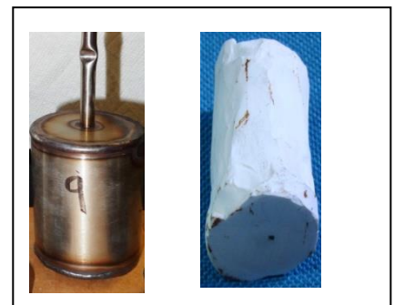
SS HIP capsule with alumina powder and Densified alumina sample after HIPing and de-encapsulation
